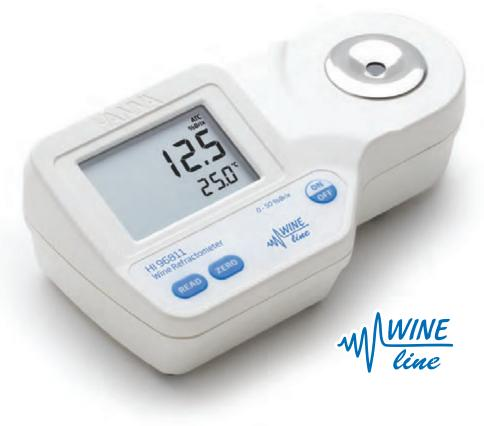
after a simple user calibration with deionized or distilled water. Within seconds, the instrument measures the refractive index of the grape must. These digital refractometers eliminate the uncertainty associated with mechanical refractometers and are ideal for fast, reliable measurements.
