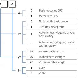
$z\!=\!1$  is supplied with 115V AC to 12V DC Adapter  $z\!=\!2$  is supplied with 230V AC to 12V DC Adapter
