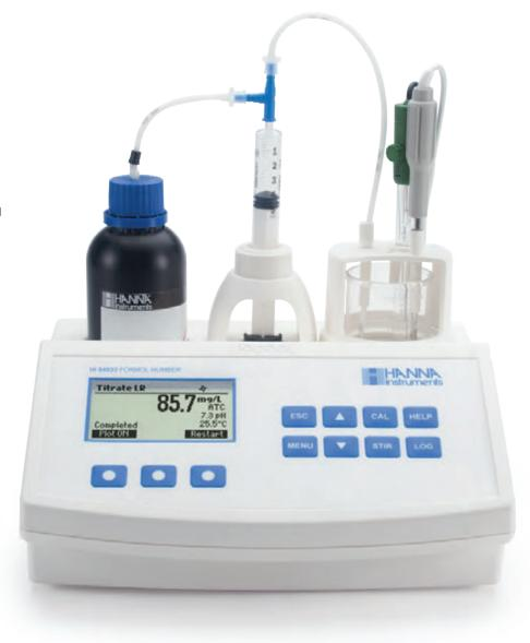
This mini titrator includes a user adjustable programmed analysis method designed for formol number analysis. It employs a powerful and effective algorithm to analyze the pH response to determine the exact pH endpoint, then uses this algorithm to perform the necessary calculations.
