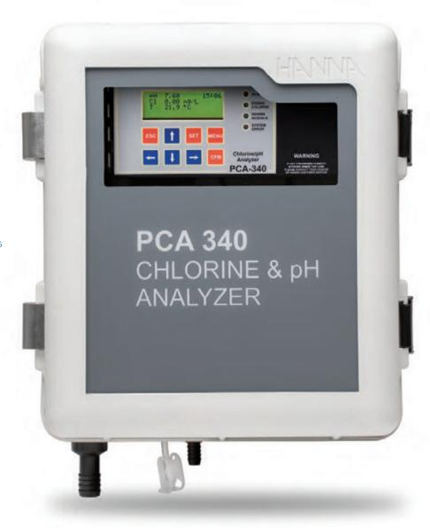
The PCA family are process analyzers for the continuous measurement of chlorine, pH (PCA320, PCA330, PCA340 only) and temperature. These analyzers feature built in data logging, RS485 digital output, dosing relays, and alarm relays packaged in a wall mount Nema 4x enclosure. The PCA340 also features two analog outputs.
