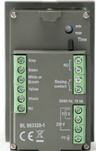
HI983320-1 rear connections example shown
