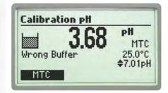
Wrong Buffer – The pH reading is not within range of the selected buffer.
